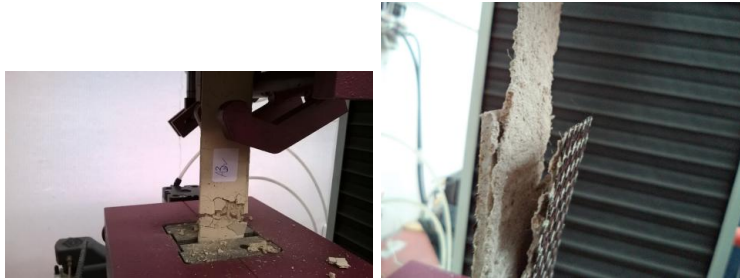
(a) Fabric failure
