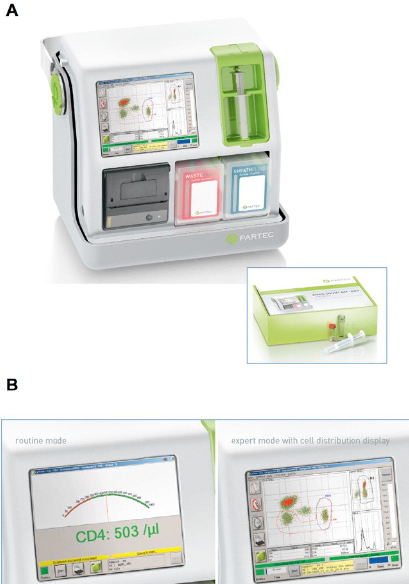
Figure 8. Partec CyFlow MiniPOC. The Partec CyFlow MiniPOC counting device (A) and its display (B) in routine (left) or expert mode (right). Both images are used with permission of Partec/Sysmex GmbH, Germany.
