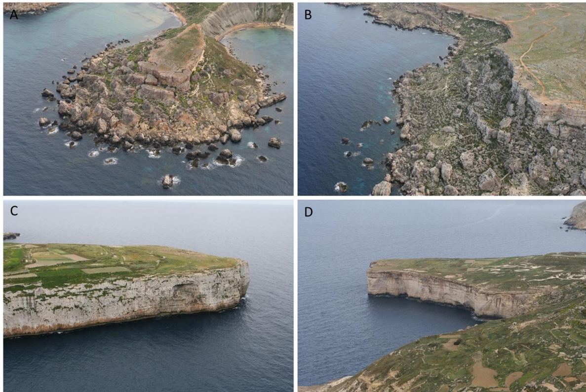
Figure 2. Rock spreading and block sliding north of Victoria Lines fault (A, B) and Lower Coralline Limestone cliffs southward (C, D).
