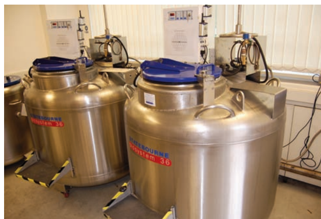
Figure 2. Cryo-storage in liquid nitrogen tanks [photo by kind permission of CABI Microbial Service (Egham, Surrey, UK)].
