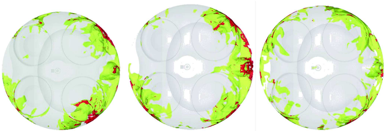
Figure 18. Combustion development and autoignition areas at +30CA ATDC for High Increase SA: Cycle A (left), Cycle B (middle), Cycle C (right).
