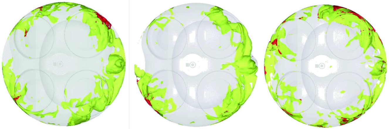
Figure 17. Combustion development and autoignition areas at +30CA ATDC for Moderate Increase SA: Cycle A (left), Cycle B (middle), Cycle C (right).
