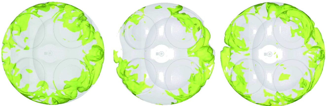
Figure 16. Combustion development and autoignition areas at +30CA ATDC for Experimental SA: Cycle A (left), Cycle B (middle), Cycle C (right).
