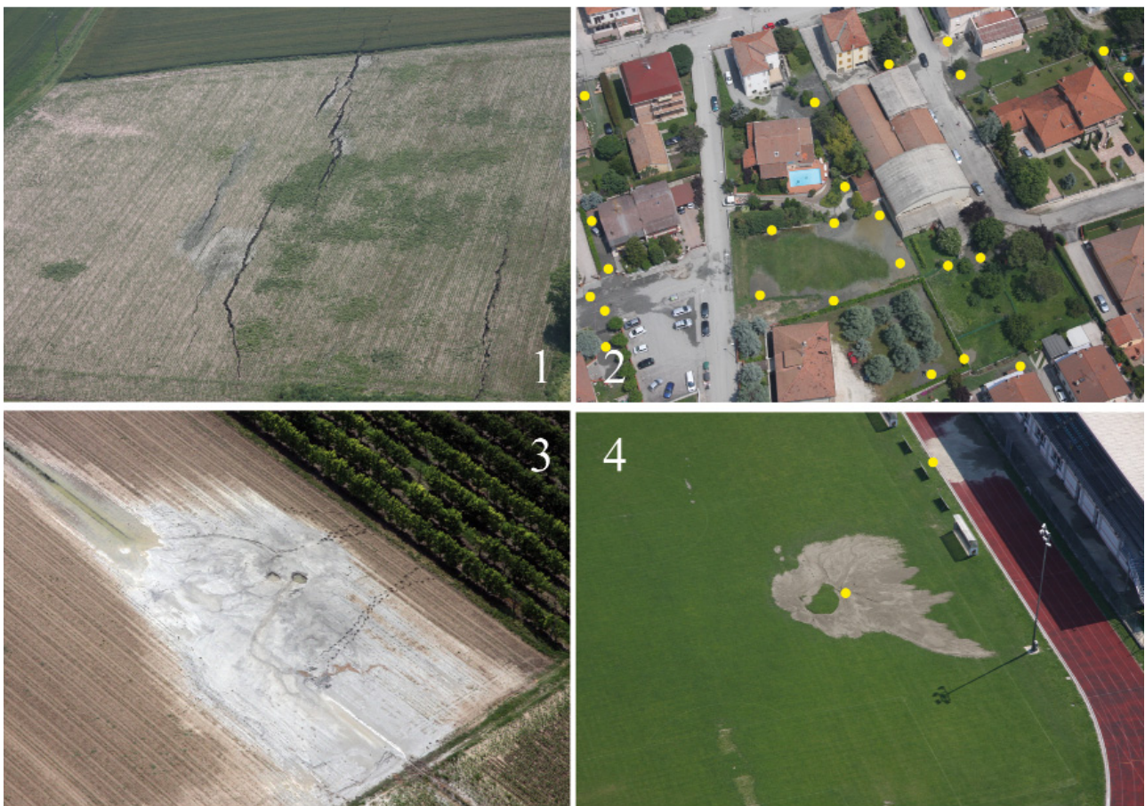
Figure 3. Some examples from the mapped surficial effects. 1) Long tension cracks (up to 1 m in width and 2 m in depth) and 'graben' south of San Carlo (Ferrara Province); 2) Sand eruptions (yellow spots) from wells, cracks and foundations inside the town of San Carlo; 3) eruption of sand in an open field; note the formation of small craters; and 4) eruption of sand in San Felice sul Panaro football field (Modena Province).
