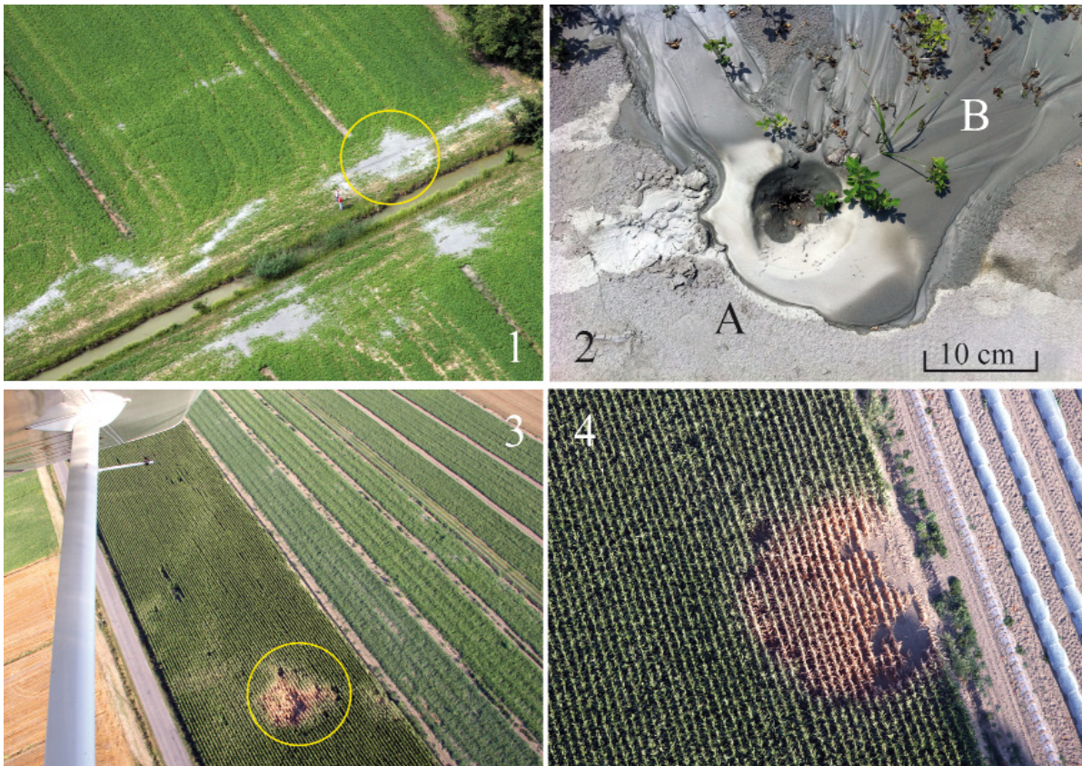
Figure 5. 1) Several 'sand volcanoes' near San Martino Spino (Modena Province). 2) Vertical close-up detail from panel (1) (yellow circle): the 'new' mud (B) erupted after the May 29 mainshock covered the sand (A) that erupted on May 20. 3), 4) Evidence of effects of dubious origin in corn plantations near Medolla (N 44.85°; E 011.08°), near to the May 29 epicenter.
