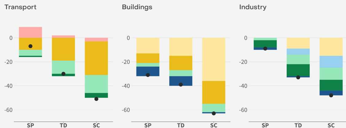
Figure 4.2.2: Reductions in estimated primary consumption of fossil fuels in modelled pathways by 2030 (difference from 2019), by the cause of reduction. The energy savings (or activity) category captures the effect of changes to consumption, before the impact of switching to more efficient end-uses (e.g. electric heat pumps). Both energy savings and efficiency improvements are considered before the impact of fuel substitution with electricity (direct electrification) or hydrogen and hydrogen-derived fuels (indirect electrification). The other category includes changes in consumption of fuels other than fossil fuels, hydrogen, or hydrogen derived fuels, for example, renewable heat and bioenergy.
