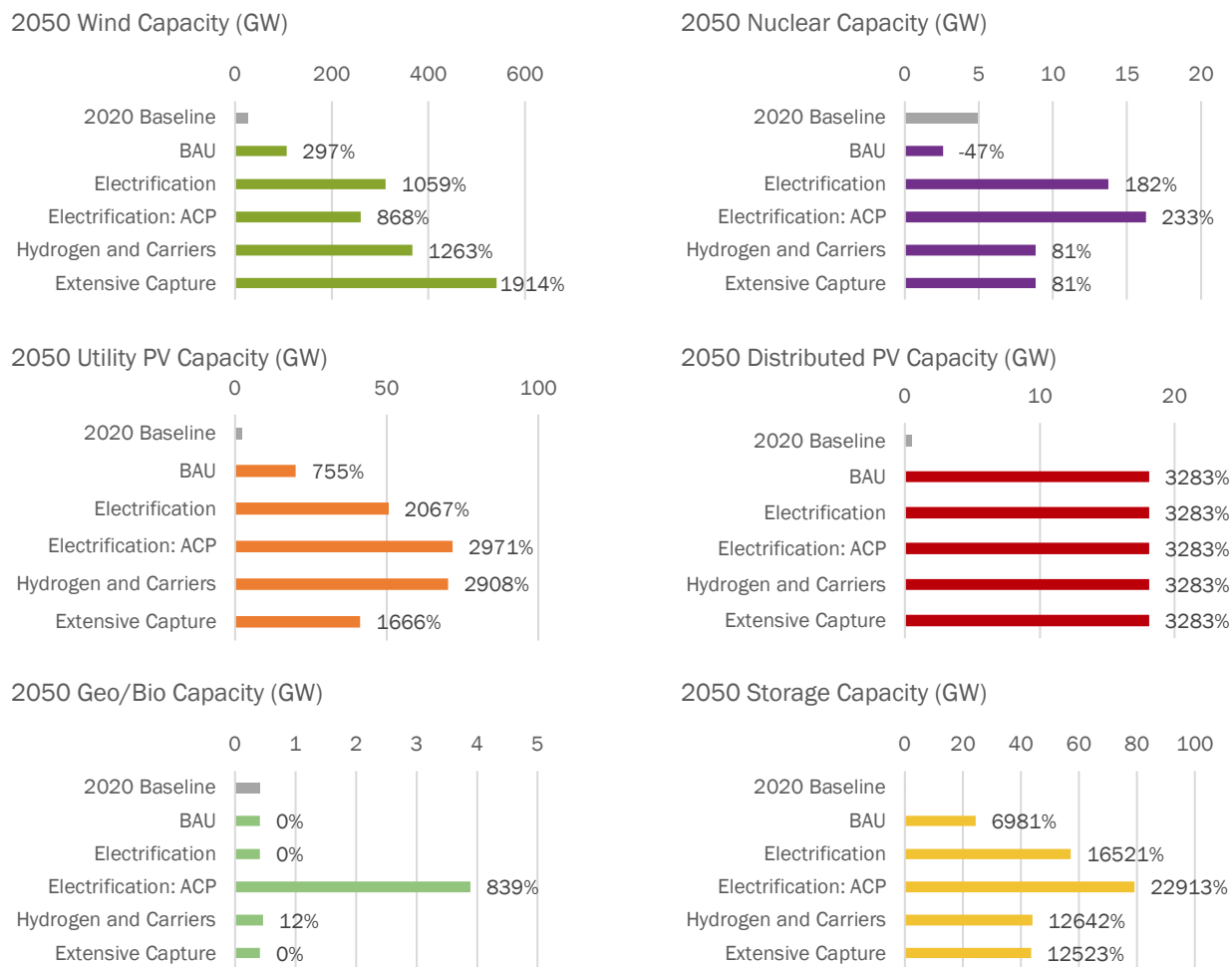
Figure 3.6: This plot shows the changes in resource capacities out to 2050 for all five scenarios, with 2050 capacity compared to the 2020 historical baseline for onshore wind, nuclear (both conventional and SMR), utility-scale photovoltaic (Utility PV, or UPV) solar, distributed photovoltaic (Distributed PV, or DPV) solar, geothermal and biomass (Geo/Bio), and storage. Nuclear, storage, and all renewables see strong growth in each net-zero scenario. The exception is geothermal, which only sees substantial capacity growth in the Electrification: Accelerated Clean Power scenario, where it is used to support a zero-carbon grid with firm generation. The zero-carbon grid is also why the same scenario sees the highest growth in storage capacity. The growth in distributed solar is equivalent between all scenarios because Distributed PV achieves optimal growth in Texas under BAU conditions; there is higher utility-scale demand in the net-zero scenarios, prompting the model to install more utility-scale resources rather than distributed. Nuclear capacity grows in all net-zero scenarios. The 2020 storage baseline is less than 0.5 GW.
