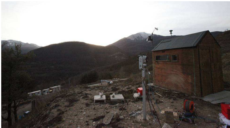
Figure 2: Photograph of the master station of the monitoring system. It shows the RTS, GNSS, meteorological station and long range TLS on the forced centring aluminium pillar.
