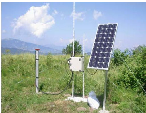
Fig.11: GPS rover (left) and its displacements in N,E coordinates (right)
