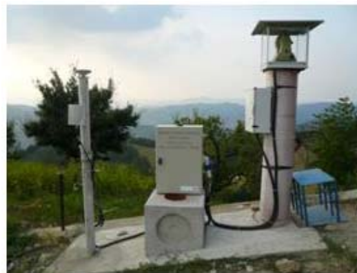
Fig. 3: Master unit composed by GPS (left) and robotic station (right)
