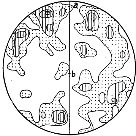
FIG. 43. 300 c-axes of quartz in the quartzofeldspathic veins of Sp. 58021501. Contours: 4-3-2-1%.
