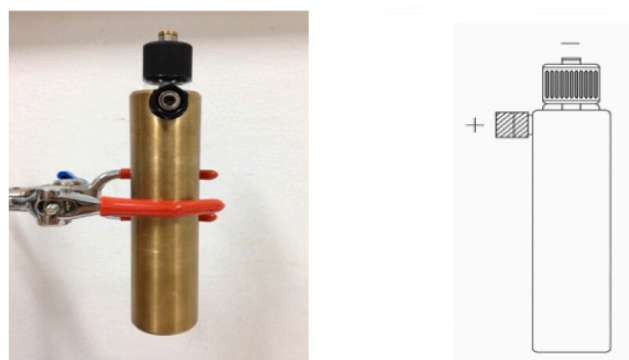
Fig. 2. Schematic representation of a pulse electric field treatment chamber (Drosou et al., 2017).
