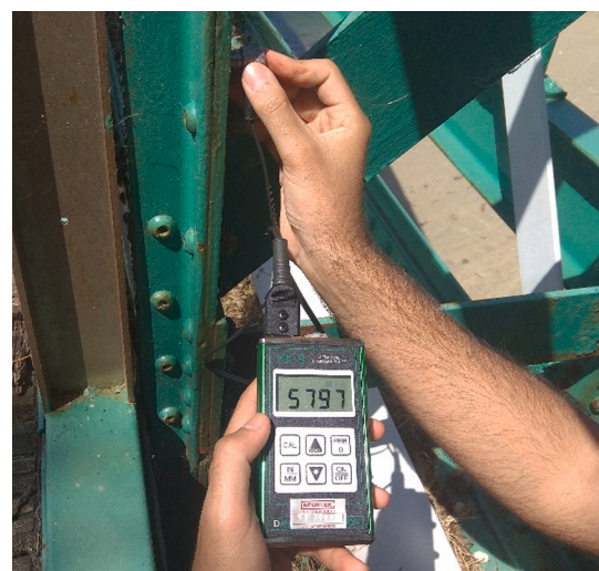
Fig. 10. Ultrasonic testing: measurement of the velocity of propagation of the longitudinal waves.
