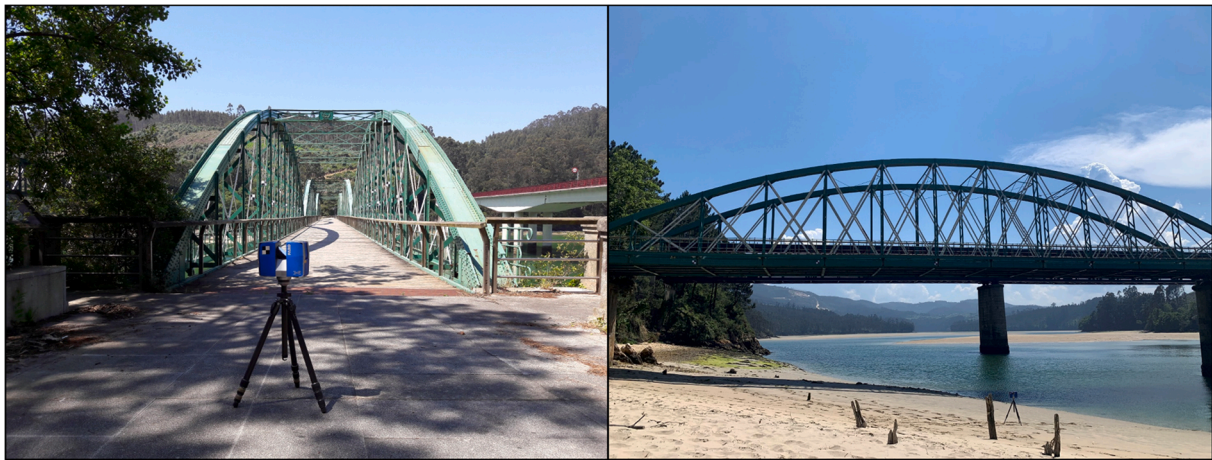
Fig. 8. Geometry data acquisition using Terrestrial Laser Scanner (TLS) technology.
