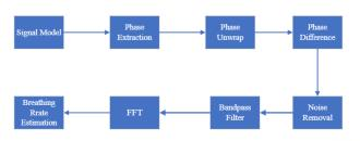
Figure 1 Block Diagram of Vital Sign Estimation
