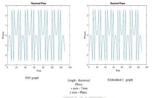
Figure 4 Received Phase for 20 BPM
