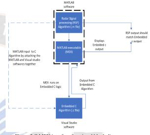
Figure 3 C MEX interface functional block diagram
