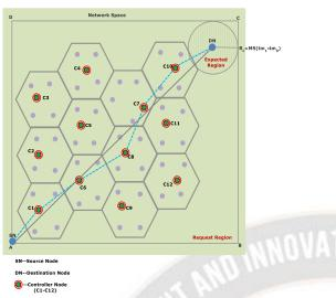
Figure 5. LAR Implementation with Honeycomb Structure
