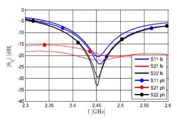
Fig. 4. Simulated S-parameters of the dual-mode antenna in free-space (fs) and on the phantom (ph).
