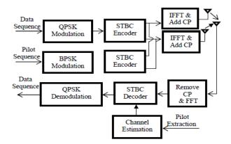
Figure 1 Block diagram of an STBC-OFDM system model.
