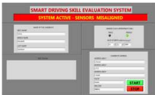
Fig 16: Graphical user Interface with misaligned sensor status after submission
