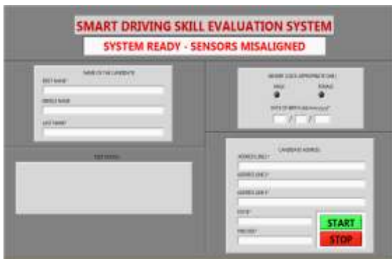
Fig 15: e-application GUI when sensor(s) misaligned
