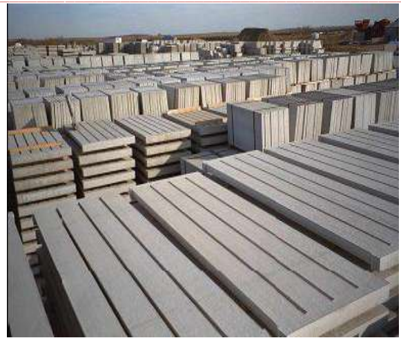
Figure 2 Manufacturing of Precast members in bulk [14]
