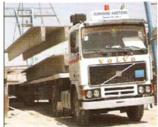
Figure 3 Manufacturing of Precast members are transported to site for assemble [14]
