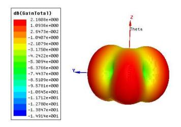
Fig:7 3D Gain Plot For Etched AMM Inclusion Antenna
