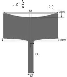
Fig:2 Y-Shaped Antenna without etched AMM Inclusion
