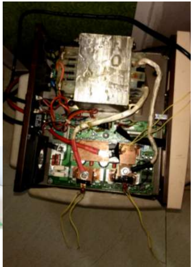
Fig 26 : Complete view showing “PTC-Cu & Cu Heat Exchanger” attached to the inverter’s PCB board.
