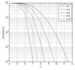
Figure 5: PAPR of OFDM signal, when N=128
