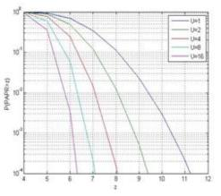
Figure 4: PAPR of OFDM signal, when N=64
