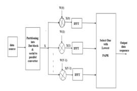
Figure 2: BLOCK DIAGRAM OF SLM METHOD
