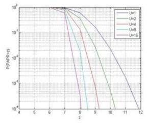
Figure 7: PAPR of OFDM signal, when N=512
