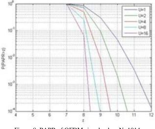
Figure 8: PAPR of OFDM signal, when N=1014.
