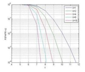
Figure 6: PAPR of OFDM signal, when N=256Figure 6 shows the plot between CCDF and PAPR it can be shown that PAPR is fall to 7.5db. It is also seen that the power saving is up to 2.5db, when N = 256.
