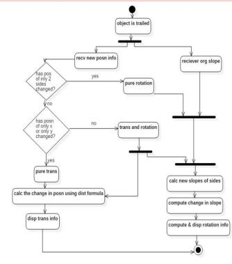
Figure 5 activity diagram for translation and rotation computation of a triangular object
