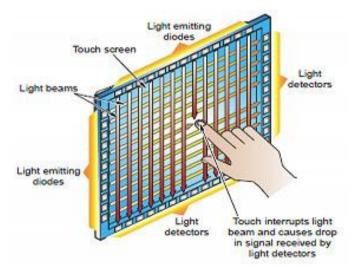
Fig 2. Working of an infra-red touch surface
