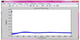
Figure 5.11: Impulse response for Chebyshev type-1 filter with 12<sup>th</sup> orders
