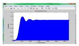
Figure 5.8: Step response for butter worth filter output with low frequency
