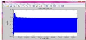
Figure 5.12: Step response for Chebyshev type-1 filter with 12<sup>th</sup> orders
