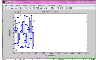
Figure 5.15: Impulse response for Elliptic filter with 12<sup>th</sup> orders
