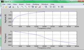
Figure 5.5: Frequency response for butter worth filter output
