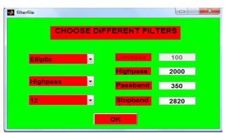
Figure 5.13: Elliptic filter with high pass frequency and 12<sup>th</sup> order
