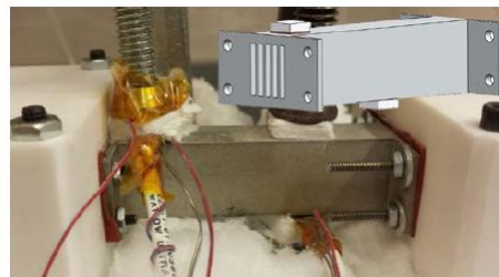
Fig. 2. Baseline aluminum sub-module test section. Ceramic resistance heaters providing the heat load are located on the top left and bottom right of the test section. Air flows from left to right.
