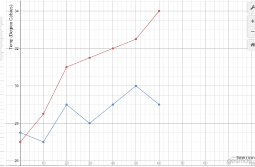
Fig 20: C3 temperature during “Al” heat sink (red) & “Cu” Heat sink (blue)
