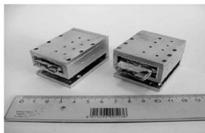
Fig 3 : Extreme left :Photograph of the two structures. Left: indirect heat removal; right: direct heat removal. Extreme right : Indicates heat flow path.
