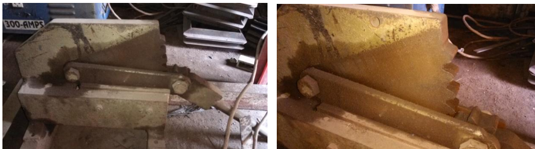
Fig 10: Left : Complete View Of The Manually Controlled Corrugated Machine. Right : Triangular Press Region Of The Machine.
