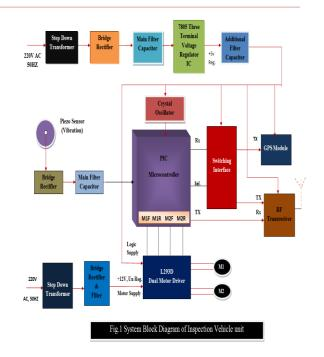
Fig .1.1 System Block Diagram of Inspection Vehicle Unit
