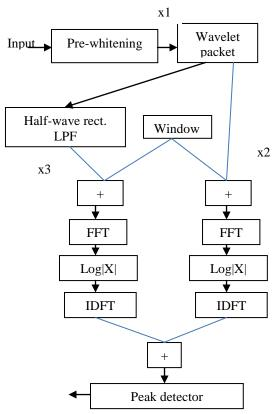
Figure.3: Block diagram of proposed pitch estimation method
