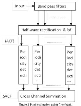
By using the spectral smoothness principle a model is proposed by Anssi P Klapuri for the determination of pitch. Here assumes the spectral envelopes of real sounds are continuous. The smoothing operation corrected approximately half of the pitch errors that occurred in a system. By using spectral smoothness principle the spectral components of a source can be separated from the mixture. Now the multipitch estimation is reduces to single pitch estimation.
