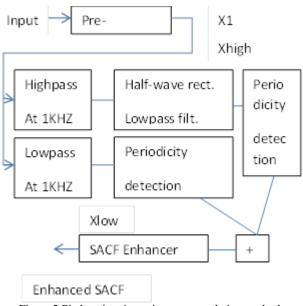
Figure.2:Pitch estimation using autocorrelation method
