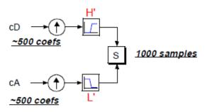
Figure 3 Wavelet Reconstruction: Approximation and Detail coefficient.
