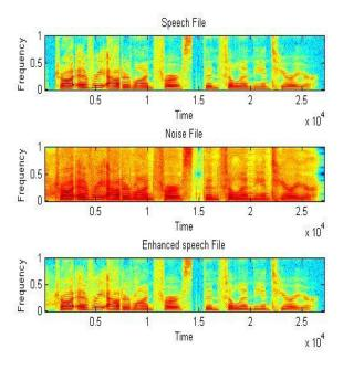
Fig 9 Signal Spectrogramplot at 15 dB babble Noise
