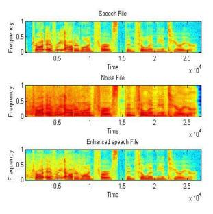
Fig 8. Signal spectrogram at 10 db babble noise
