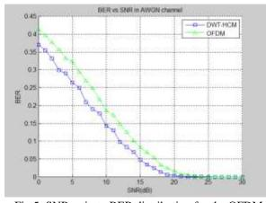
Fig 5: SNR ratio to BER distribution for the OFDM and DWT-HCM Transform modulation
