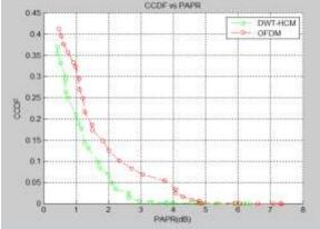
Figure 4: PAPR to CCDF distribution for the OFDM and DWT-HCM Transform modulation.
