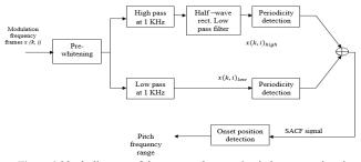
Figure.2 block diagram of the proposed system's pitch range estimation method
