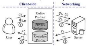
Fig. 1. System architecture of UPS.
