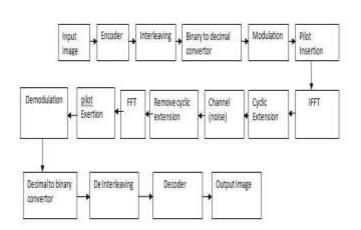
Figure 1: Block Diagram of OFDM Transceiver System
