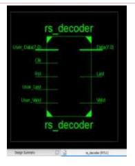
Fig.5 RTL view of RS Decoder showing input and output port
