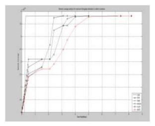
Figure 12:- Graph in between data rate and network coverage for uniform Scenario
