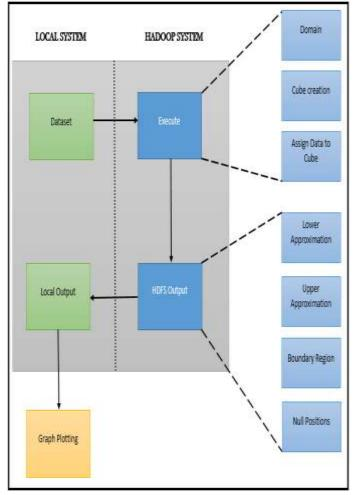
Figure 1: System Architecture
