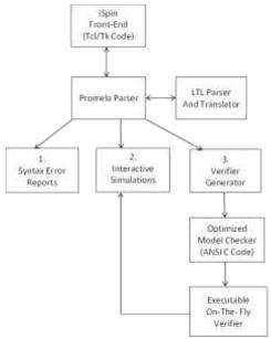
Fig. 2 Basic structure of SPIN [6]
