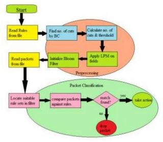
Figure 5. System flow architecture
