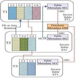
Fig. 4. Management of the encryption keys according to the field confidentiality parameter.
