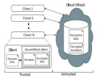
Fig. 1. SecureDBaaS architecture.
