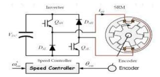
Fig.1 SRM with one phase asymmetric converter
