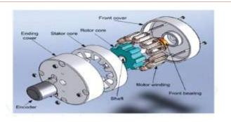
Fig.3. Construction diagram of SRM
