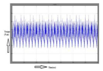
Fig. 23 Toque waveform with FLC-PI controller
