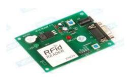
Figure 4. 125KHz RFID Reader Module
