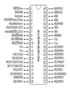
Figure 2. Pin Diagram of PIC16F877A
