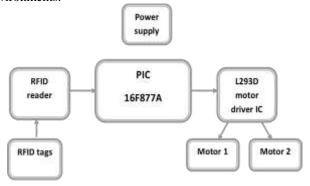
Figure 1. Schematic of the Project
