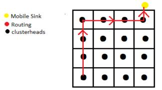
Fig 1. VGDRA approach showing straight line communication.
