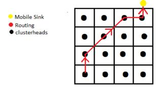
Fig 2. Proposed approach showing the selection of cluster head on the basis of shortest distance between next clusters choosen for communication or the nearest cluster.
