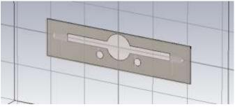
Figure 4: Back View of Proposed 4th order HPF using DGS.
