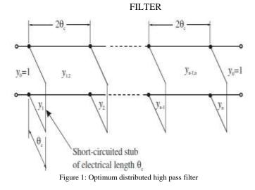
The proposed high pass filter (HPF) consists of shunt short circuited stubs of electrical length  $\Theta c$  at some specified frequency fc (usually the cut off frequency of HPF). These elements were separated by unit elements (UE) of length  $2\Theta c$  shown in the figure 1 [12]. In theory this type of filter has very wide band response for small  $\Theta c$  but this requires a high value of impedance in the short circuited stub (SC-Stub).
