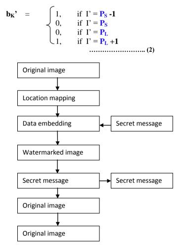
Fig.1. Procedure of the proposed algorithm.
