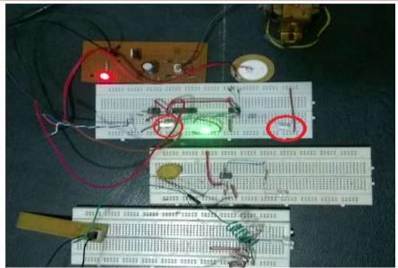
Figure – 7 Hardware Implementation of Sensor And IR Transmitter.
