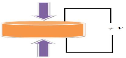
Figure.3. piezoelectric pressure sensor
