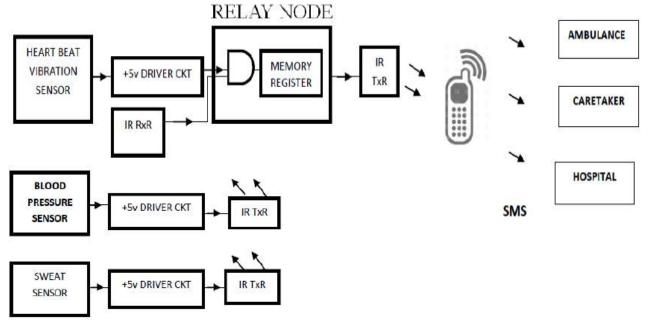
Figure – 6 Block diagram of secure IR module.
