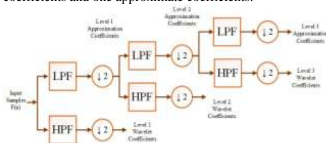
Figure 2. Three stages in Forward Discrete Wavelet Transform decomposition
