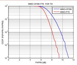
FIG 5 .PAPR reduction in MIMO-OFDM with PTS
