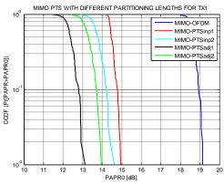
Fig6: PAPR reduction of MIMO-OFDM with different partitioning techniques and PTS
