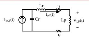
Fig. 4. Equivalent circuit before lamp ignition
