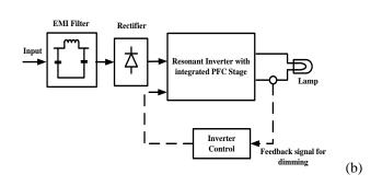
Fig.1. Typical electronic ballast systems. (a) Two-stages ballast circuit. (b) Single-stage electronic ballast.
