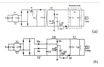
Fig. 2. Derivation of proposed ballast circuit. (a) Existing circuit (b) Derived circuit.
