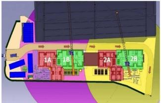
Fig. 5. The location of the two tower crane and the four bays
