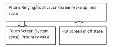
Figure 3. .Close environment Control flow
