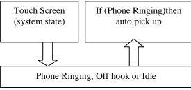
Figure 2. Automatic call picker Control flow
