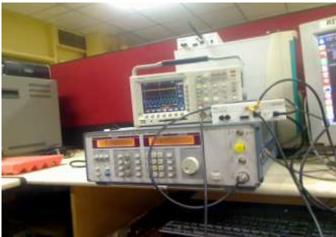
Fig. 7: DDC to DUC loopback system
